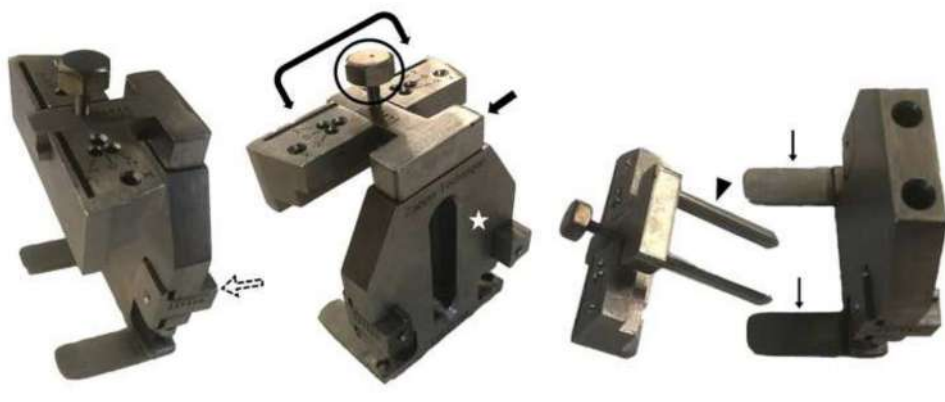
Fig. 2 The newly introduced guide for femoral cutting during TKA. Asterisk: the base; thick arrow: mounting mechanism; thin arrows: projections; dashed arrow: spacer; double arrow: cutting guide; arrowhead: rod; circle: screw tight fastener
